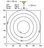
Light sourceLEDWork equipmentWithoutConnected load22 - 26 V; DCPower consumptionca. 25 W
